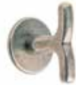
GAS VALVE COVER PART # GVC | SIZE Ø2 3/8" x 3 1/8" Shown in silicon bronze medium patina. Includes 12" extension with 5/16" square adapter. See page 164-170 for additional handle options.
