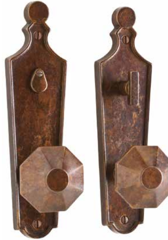
ESCUTCHEON 2 1/2" x 9 1/4" FUNCTION PRIVACY MORTISE BOLT/ SPRING LATCH KNOB K10015 OCTAGONAL PATINA SILICON BRONZE RUST PART # E10017/E10016
