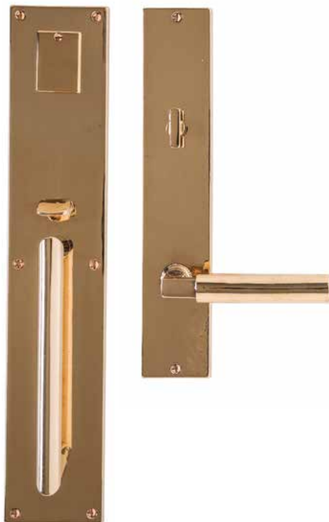
ESCUTCHEON 3 1/2" x 18" | 2 1/2" x 13" FUNCTION ENTRY THUMBLATCH MORTISE LOCK GRIP | LEVER G365 JANE & L154 STALK PATINA SILICON BRONZE HIGH POLISHED PART # G206/E257
