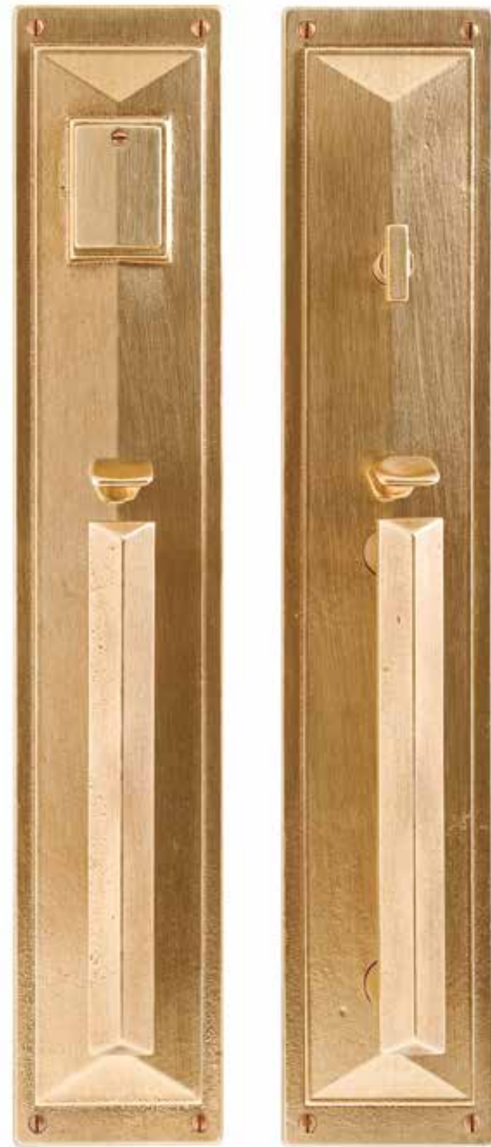
ESCUICHEON 3 3/4" x 20" FUNCTION ENTRY THUMBLATCH MORTISE LOCK GRIP G21075 7 1/2" MACK PATINA SILICON BRONZE BRUSHED PART # G21033/G21031
