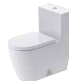
Set Toilet One-Piece Duravit Rimless® elongated with syphonic jet action, 305 mm/12" rough-in, with dual flush piston valve, top flush, vertical outlet. One-Piece Toilet incl. seat & cover w/ soft closure
